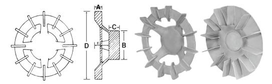
**DIMENSIONS** Overall diameter (D) is most critical in determining air delivery over the motor. Blade width or height (A) is also important, but the number of blades is not significant. Be sure the fan blade you choose clears the bearing housing outside diameter, and the fan cover inside diameter. Tolerances are  $\pm$  1/8" on all dimensions except bore.
