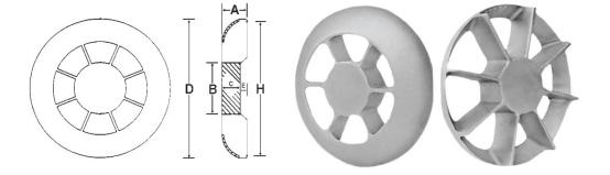
**DIMENSIONS** Overall diameter (D) is most critical in determining air delivery over the motor. Blade width or height (A) is also important, but the number of blades is not significant. Be sure the fan blade you choose clears the bearing housing outside diameter, and the fan cover inside diameter. Tolerances are  $\pm$  1/8" on all dimensions except bore.
