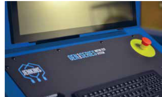
Separate Operator Console allows the user to energize the motor under test and monitor live data at a safe distance.
